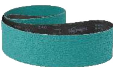
High-quality zirconium grain and strong polyester cloth backing. The active add-on layer (TOP SIZE) improves stock removal performance, prevents clogging, and allows for cooler grinding. Ideal for high carbon and alloy steel and stainless steel.
