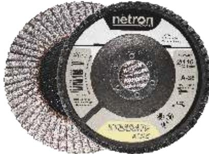
It is designed to prevent clogging that may occur on the disc surface in aluminum and similar soft metals. The Calcium Stearate coating on the abrasive surface liquefies under heat and does not fill the disc surface, maintaining the high cutting rate of the disc and ensuring long working life. It is perfect for aluminum, bronze, copper, and similar soft metals.
