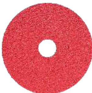
The multi-layer fiberglass backing and the continuously self-sharpening ceramic grain offer intensive stock removal performance and long working life. An additional top coating (TOP SIZE) makes colder grinding possible, preventing discoloration on workpiece surfaces.
